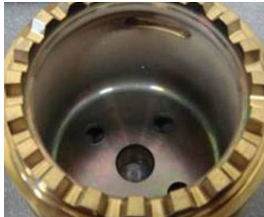
Hollow shaft at 1500 hours with IBF installed
