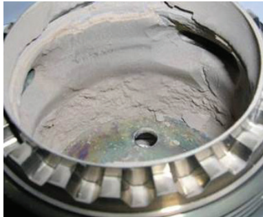
Hollow shaft at 800 hours with no IBF
